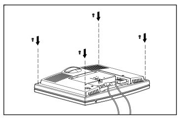
Figure 2-18. Inserting the monitor case screws
